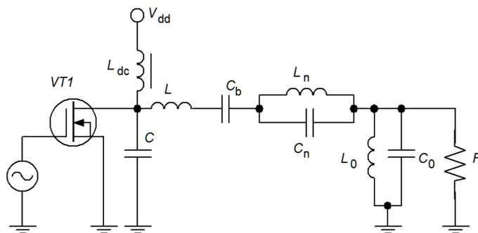
*Fig. 1. Class-EF power amplifier schematic*
