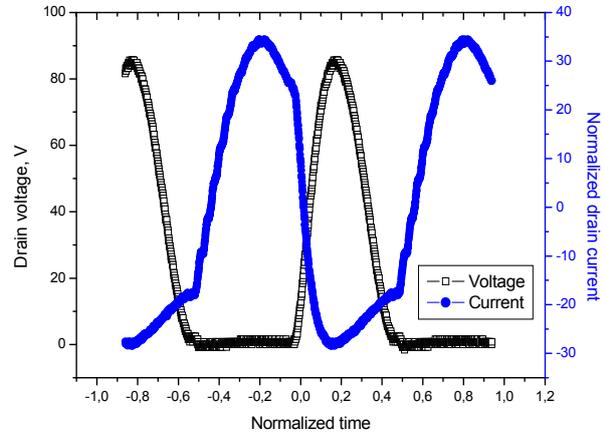
Fig. 5. Drain voltage and current waveforms for  $C_n=864$  pF
